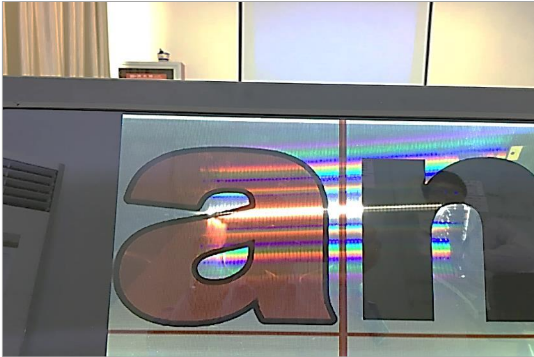
Reflector Panel deactivated TFT background is transparent
