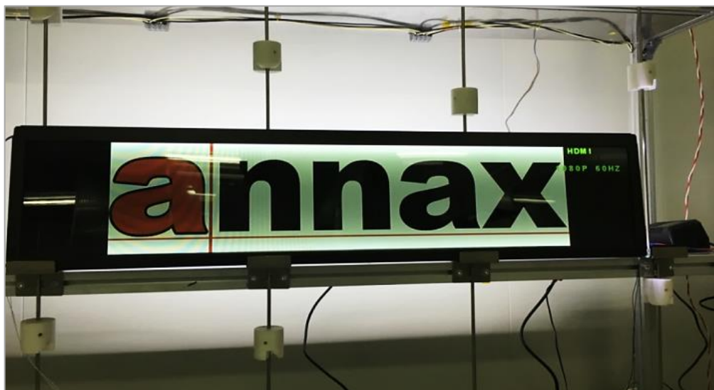
Front view – TFT and reflective panel active
